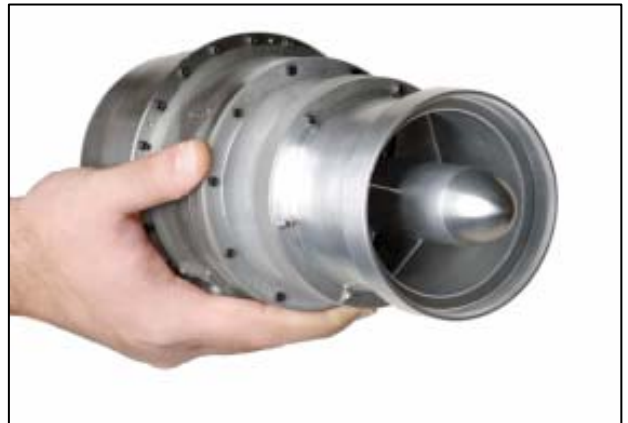
FTT's small turbofan, FTA37F, fits in the palm of your hand but is designed to power small unmanned air vehicles over long ranges.
